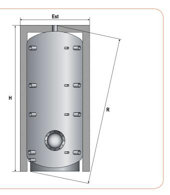
TA - TAS tanks are designed to be operated in conjuction with a plate heat exchanger to generate domestic hot water requirements.
